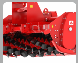
Helical Shape of Rotor Blades
