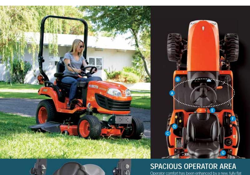
deck layout with the brake on the left side, providing more room for the feet. The new design also improves operability.
